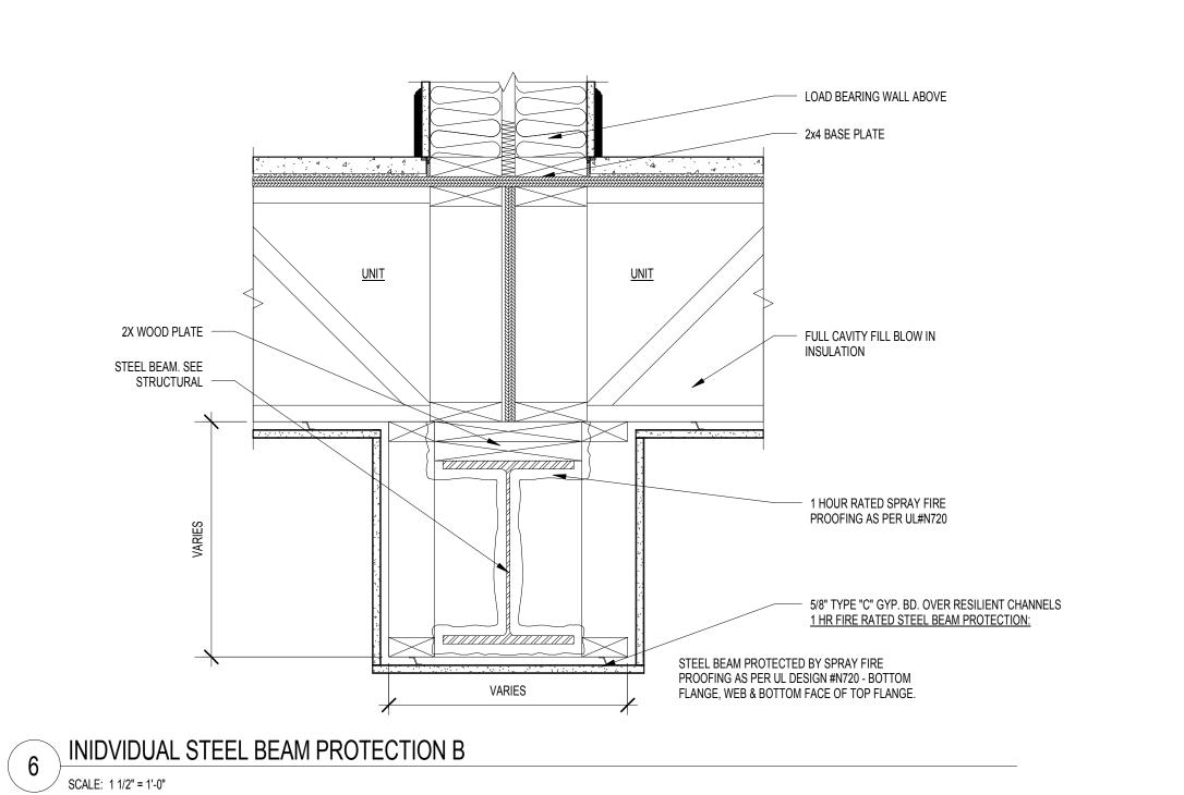
LOAD BEARING WALL ABOVE 2x4 BASE PLATE 2X WOOD PLATE 1 HOUR RATED SPRAY FIRE PROOFING AS PER UL #N720 STEEL BEAM. SEE STRUCTURAL FULL CAVITY FILL BLOWN IN FULL CAVITY FILL BLOWN IN INSULATION INSULATION -TRUSS HANGER & WOOD TRUSSES BEYOND TRUSS HANGER & WOOD TRUSSES BEYOND 1-HOUR FIRE RATED STEEL BEAM PROTECTION: STEEL BEAM PROTECTED BY SPRAY FIRE PROOFING AS PER UL DESIGN #N720 - BOTTOM FLANGE, WEB & BOTTOM FACE OF TOP FLANGE. - 5/8" TYPE "C" GYP. BD. OVER RESILIENT CHANNELS
