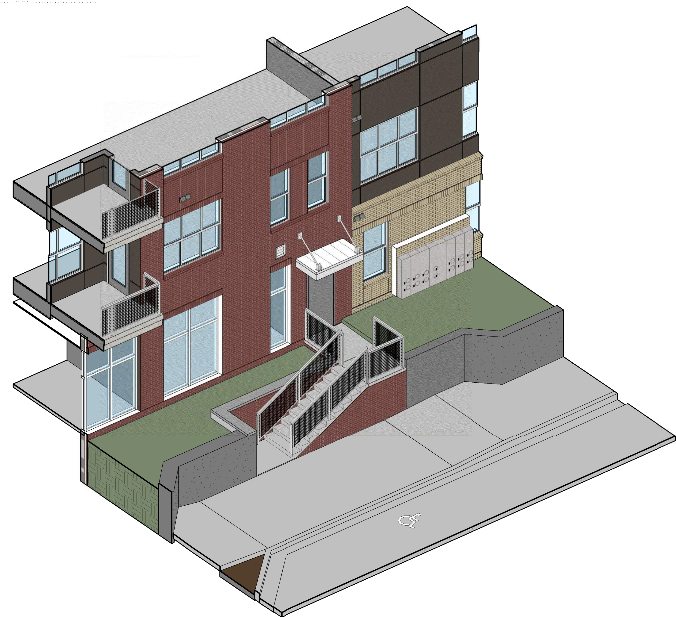
4 STAIR B EXTERIOR STAIR AXON
