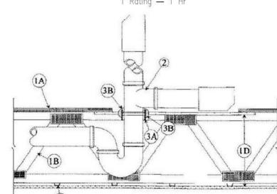
1. Floor-Ceiling Assembly — The 1 hr fire-rated solid or trussed lumber joist floor-ceiling assembly shall be constructed of the materials and in the manner specified in individual L500 Series Floor—Ceiling Designs in the UL Fire Resistance Directory, as summarized below:
