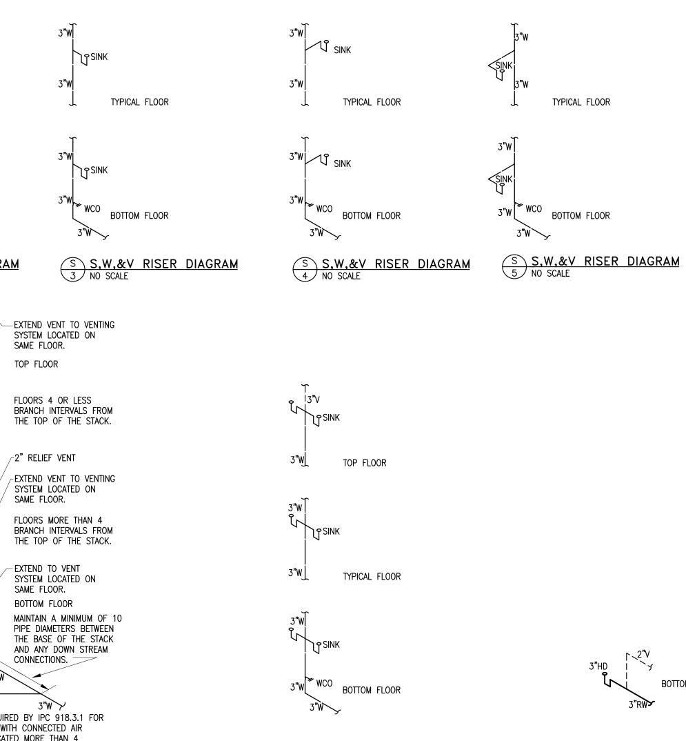
S S,W,&V RISER DIAGRAM 8 NO SCALE
