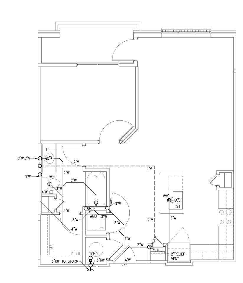
UNIT A2 BOTTOM FLOOR PLAN - S,W&V
