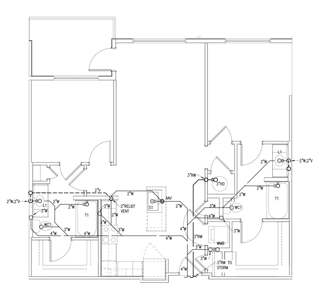
UNIT B1 BOTTOM FLOOR PLAN - S,W&V
