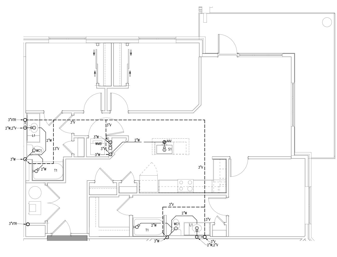
4 UNIT C1A TOP FLOOR PLAN - S,W&V SCALE: 1/4" = 1'-0"
