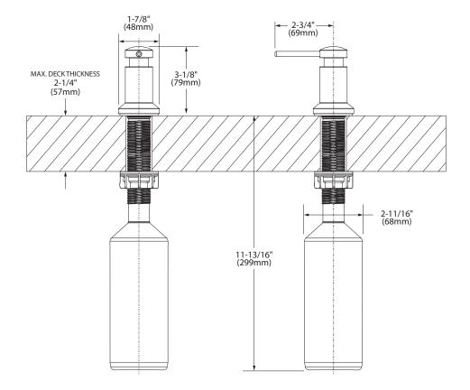
NOTE: DESIGNED TO BE INSTALLED THROUGH 1 HOLE 1-1/8" DIAMETER
