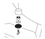
Install the washers, nuts, and caps on the flange bolts snug. Be careful not to over tighten because the china may break.
